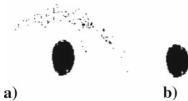
Fig. 13 Results illustrating the isolated pupil pattern. a Pupil isolated result, b Isolated pupil after enhancement
