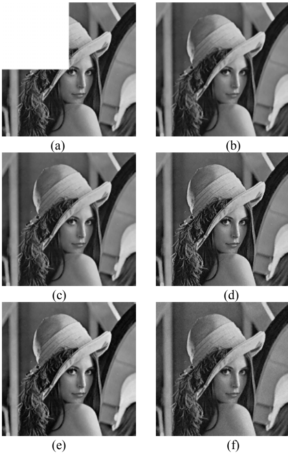
Figure 13. The spatial-domain-attacked watermarked images. (a) Image cropping in the upper-left corner. (b) Median filtering with the radius of 2 pixels. (c) Blurring with radius=1.0 and threshold=10.0. (d) Sharpening. (e) Contrast Enhancement by 10%. (f) Adding Gaussian noise by the amount of 4%.
