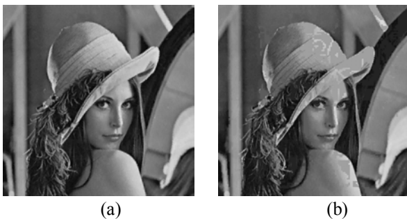
Figure 6. Watermarked images obtained by algorithms in different embedding orders. (a) Watermarked image with PSNR=30.40dB obtained by the proposed method. (b) Watermarked image with PSNR= 26.97dB obtained by the algorithm in the reverse embedding order.
