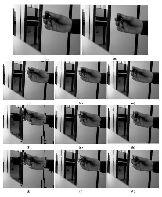
Figure 5: (a) Reference frame, (b) Current frame, (c) FS  $16 \times 16$  block, (d) FS  $8 \times 8$  block, (e) FS  $4 \times 4$  block, (f) TSS  $16 \times 16$  block, (g) TSS  $8 \times 8$  block, (h) TSS  $4 \times 4$  block, (i) FSS  $16 \times 16$  block, (j) FSS  $8 \times 8$  block and (k) FSS  $4 \times 4$  block.
