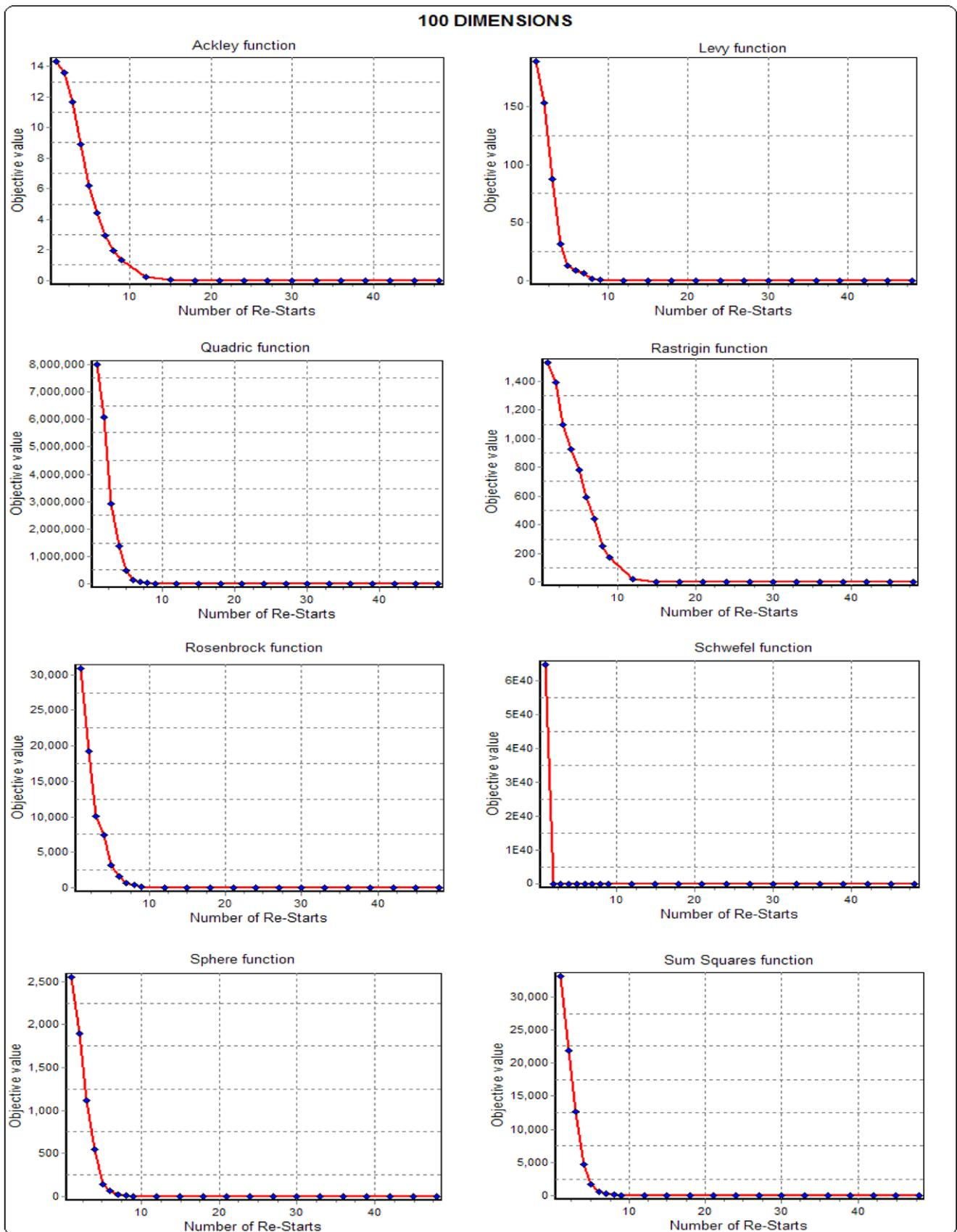
**Fig. 9** LSRS convergence for 100 dimensions
