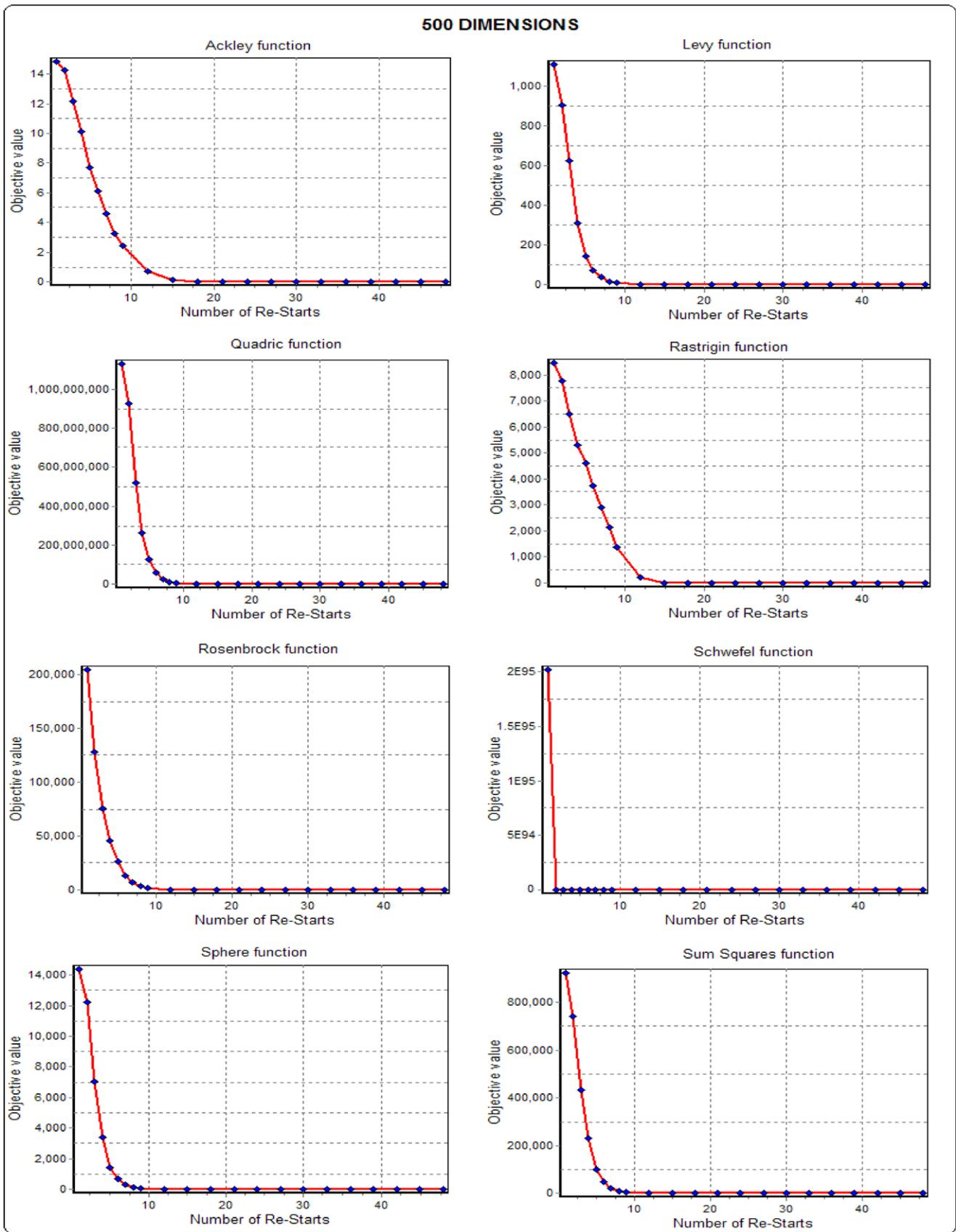
**Fig. 11** LSRS convergence for 500 dimensions
