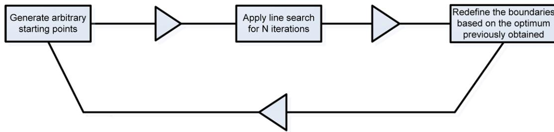
**Fig. 1** The general scheme of the LSRS
